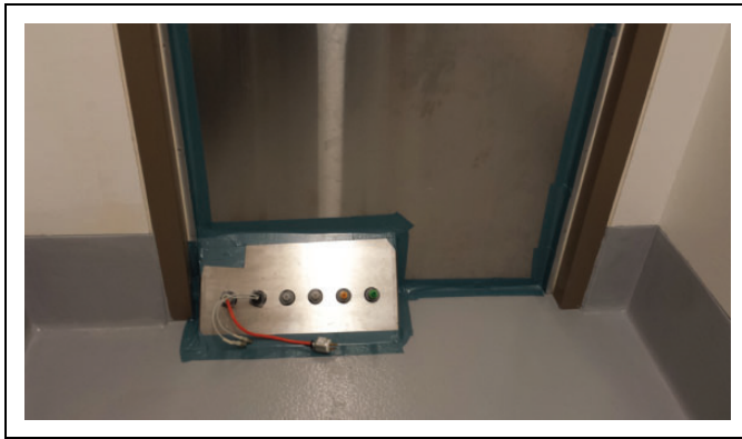
Figure 2. The Under-the-Door-Plate. This plate allows the chlorine dioxide gas generator connections to enter the room without any modification.
