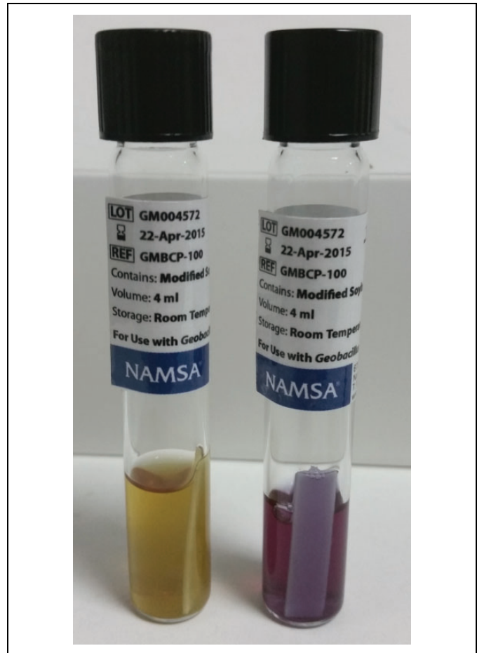
Figure 5. The incubation media tubes. The yellow tube (left) shows growth, and the purple tube (right) shows no growth.
