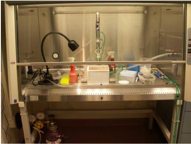
Fig. 1. Pneumatically operated cryo-plunger to vitrify samples for Cryo-EM in a BSL-3 containment of the W.M. Keck Center for Virus Imaging at UTMB. Note that the plunger is inside of a BSC to protect researchers from exposure to samples. Pneumatic cylinder, tweezers guard, container for waste with disinfectant, and other materials and tools used for freezing grids are indicated in the figure.
