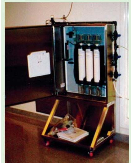
Photo 2: Prototype chlorine dioxide gas generator showing CD-generating cartridges
