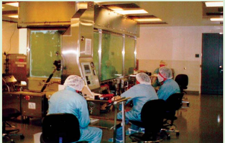
Photo 1: Aseptic fill isolator undergoing chlorine dioxide disinfection
