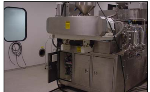
Example 1: (Blow Fill Seal Machine)
